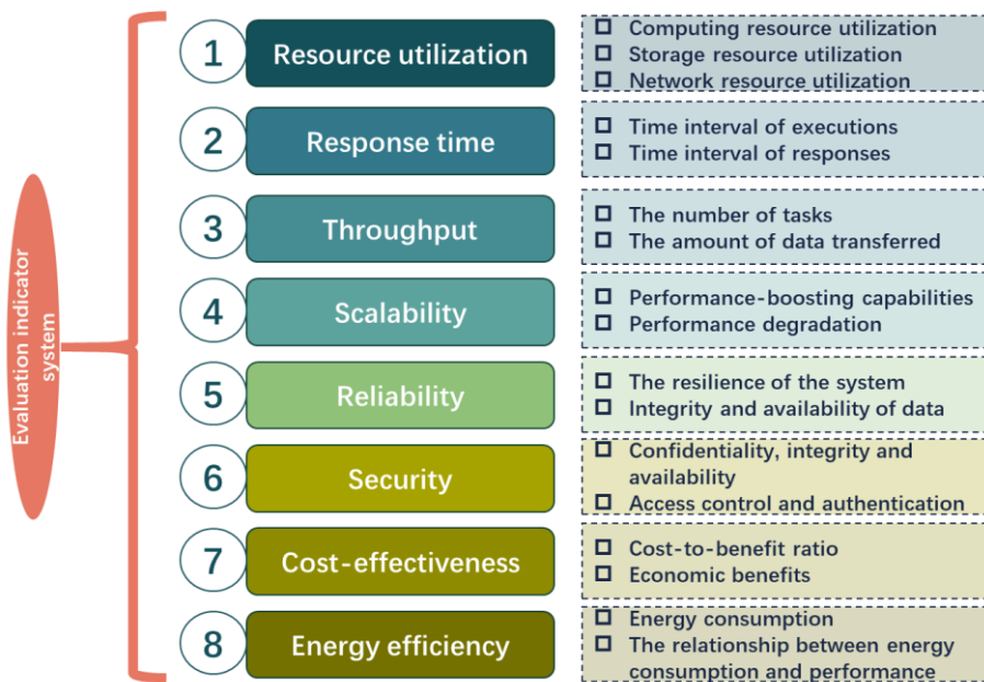
Figure 5. Indicator system for evaluating the performance of computer hardware and software resource sharing under cloud computing conditions
